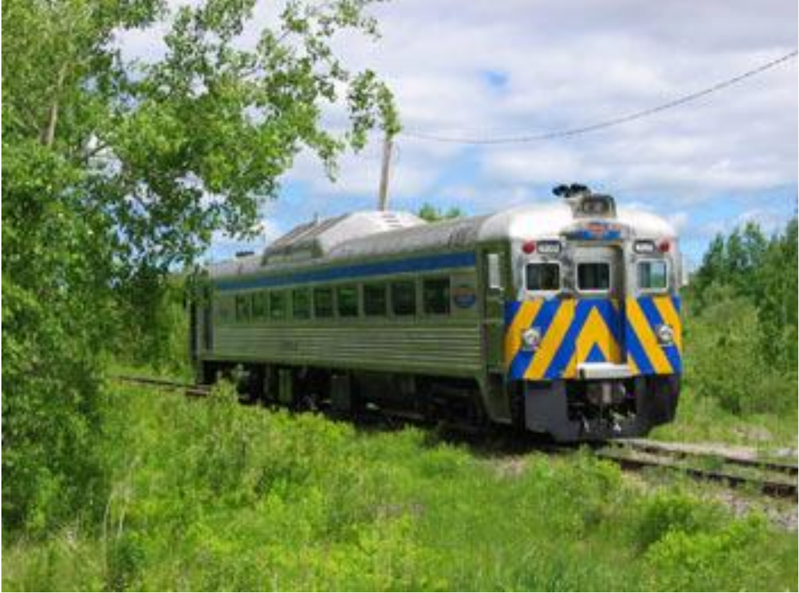
IRSI's remanufactured demonstrator RDC #6202 on a test run.
