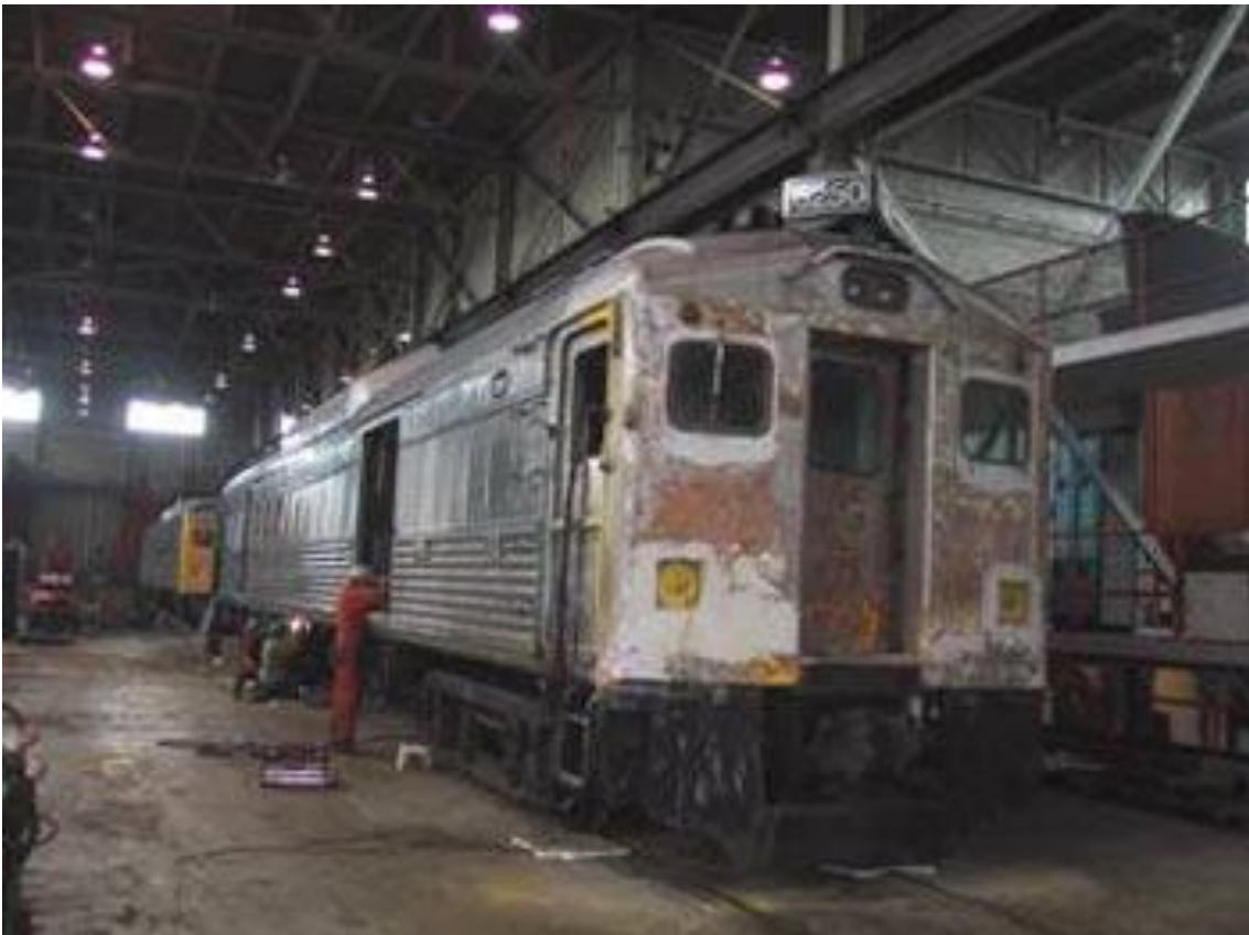
IRSI's demonstrator RDC #6202 at the beginning of the remanufacturing process.
